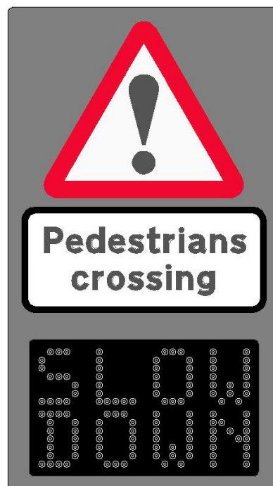
Fig1. Diag No. 562 with supplementary plate No.563. Vehicle activated panel with 'SLOW DOWN' text.
